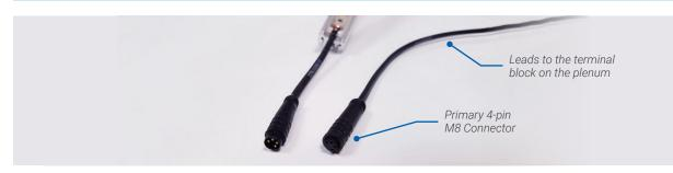
Step 2: Connect a spare functional LED to the primary 4-pin M8 connector.
