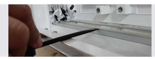
**Step 3:** To install the new LED strip, ensure the connector ends on the LED are oriented such that the male connector of one LED and the female connector of the adjacent LED align.
