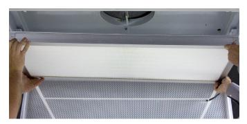
B) Ensure knife edge of plenum seats into gel channel. Use guides to assist with proper knife edge alignment.
