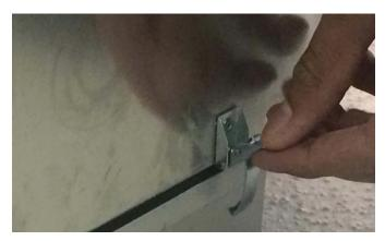
B) Attach filter to top cap assembly by hooking and securing latches. Gasket may need to be compressed to grab channel with latch.
