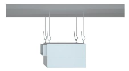
**Step 8:** Raise adjacent module assemblies, temporarily supporting the modules with hanger wire. Fasten modules together using bolts, metal washers, and lock nuts supplied by Keystone. Module sections will have slotted holes for fastening. Bottom of modules should be flush and level prior to fastening together.
