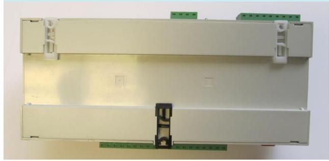
Front view of WEB-SERVER mounted on din rail
