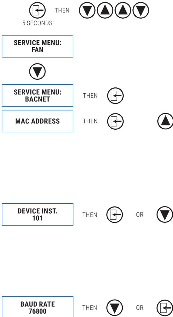
Hold down the **Menu** button on the LCD Thermostat for **5 seconds** until prompted for a passcode; use **▲** and **▼** to enter the passcode; **DOWN, UP, UP, DOWN**.
