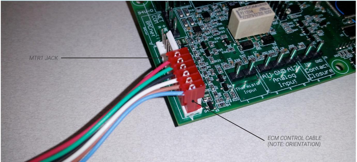
**NOTE:** Make sure that this cable is connected properly. It is keyed one way, and make sure all of the pins are covered.
