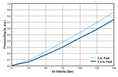
Note: Pressure drop shown is factory maximum allowable at equivalent air flow based on effective filter media area.
