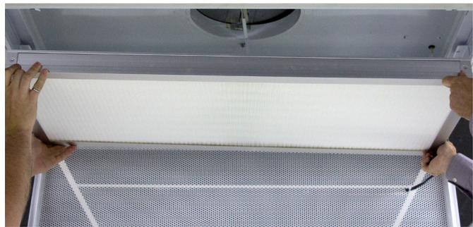
B) Ensure knife edge of plenum seats into gel channel. Use guides to assist with proper knife edge alignment.
